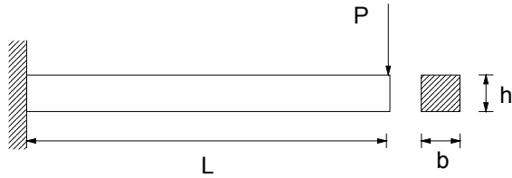
Figure 7 Cantilever Beam Problem Description
